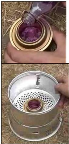
3. Assemble the burner. Remove the lid off the brass burner unit and pour in some methylated spirits. Do not overfill. Replace the lid immediately. Put the burner carefully in the centre of the wind shield and put the second wind shield in place. A few drops of water will make it easier to clean (not too much or it won't light!)
