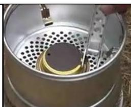
8. Finish cooking. Put the closed burner top in place to turn off the stove. The lack of oxygen will cause the methylated spirits to stop burning after just a few seconds. Do not use the burner lid to extinguish the stove, the rubber seal inside the lid is not fireproof and will burn and melt all over your burner. Remove the burner top to make sure the fire has extinguished. Leave the Trangia to cool before packing it away. Wrap the burner in the plastic bag to avoid leaks.
